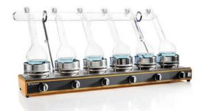
For Kjeldahl flasks of sizes 50, 100, 250, 500 and 750 ml. Each heater can be adjusted individually and continuously. With efficient glass exhaust manifold (with adapters tailored to the flask size), Kjeldahl flasks, stands and mains cable.
