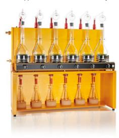
For Kjeldahl flasks of sizes 50, 100, 250, 500 and 750 ml. Each heater can be adjusted individually and continuously. With Kjeldahl flasks, Reitmair tops, condenser tubes, discharge tubes, Erlenmeyer flasks, all rubber connectors, stands and mains cable.
